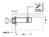
The top screw in front of the hanger adjusts the vertical movement, while the bottom screw adjusts the depth movement.
