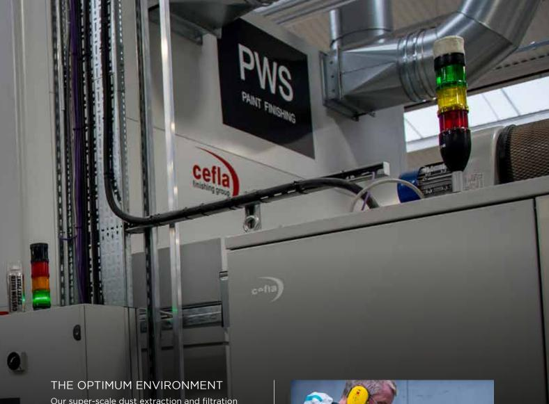
Our super-scale dust extraction and filtration network cleans the air in the whole building, every hour - to continuously ensure the purest environment and optimum paint finishing conditions.
